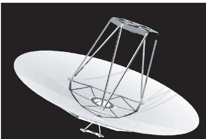
Figure 7. Assembled primary and secondary reflectors of the Herschel Space Observatory (13) .
