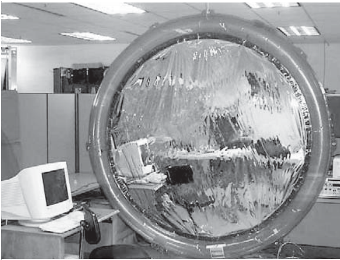
Figure 10. Alternative membrane reflector support structures: (a) Inflatable torus support (42) , (b) Discrete attachment points.
