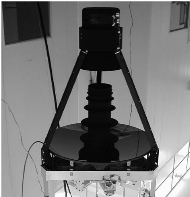
Figure 6. The Akari SiC mirror assembly (6) .
